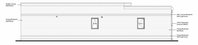
PROPOSED Block B - North West Elevation 1:100 @A3 1:50 @A1 Scale
